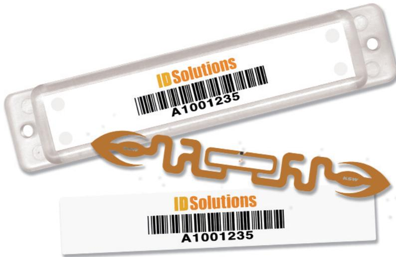
For asset tracking applications that require heavy impact or water resistance we offer our RFID Hard Tag. Constructed of durable impact resistant polycarbonate, this product features a hermetically welded housing that protects the subsurface printed label and the RFID inlay from rigorous environments. Inside the housing the air gap between the inlay and the metal surface provides for a longer read range than similar products. Affixing methods include mechanical fasteners and/or adhesive.
