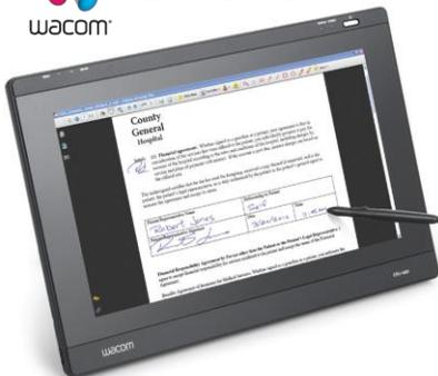
A 16" widescreen interactive pen display that is ideal for displaying entire pages of electronic documents, such as loan applications, and the pen can be used anywhere on the screen to fill in electronic forms and sign the document electronically as if it were paper. This pen display can be used in landscape or portrait orientation with the included adjustable stand or it can be mounted securely on an LCD arm and attached to the counter.
