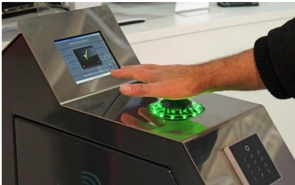
PalmSecureID with 'Magic-Eye' integrated into a turnstile
