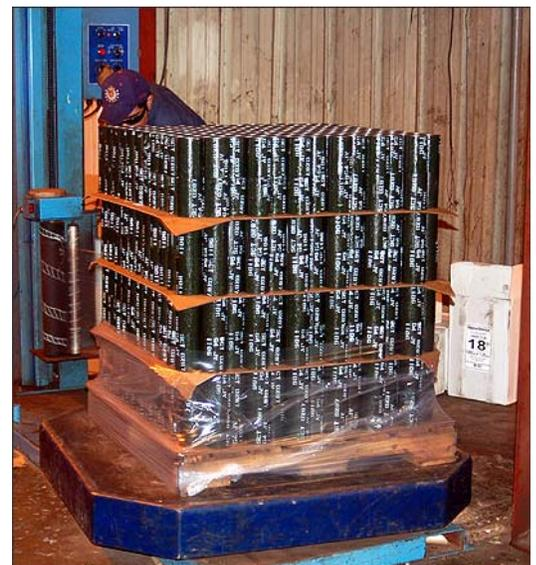
*Drill pipes and other products are shrink-wrapped and their RFID tags read*
