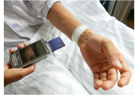
An RFID (Radio Frequency Identification) chip stores the wearer's data, which can be accessed by a hand-held computer or laptop
